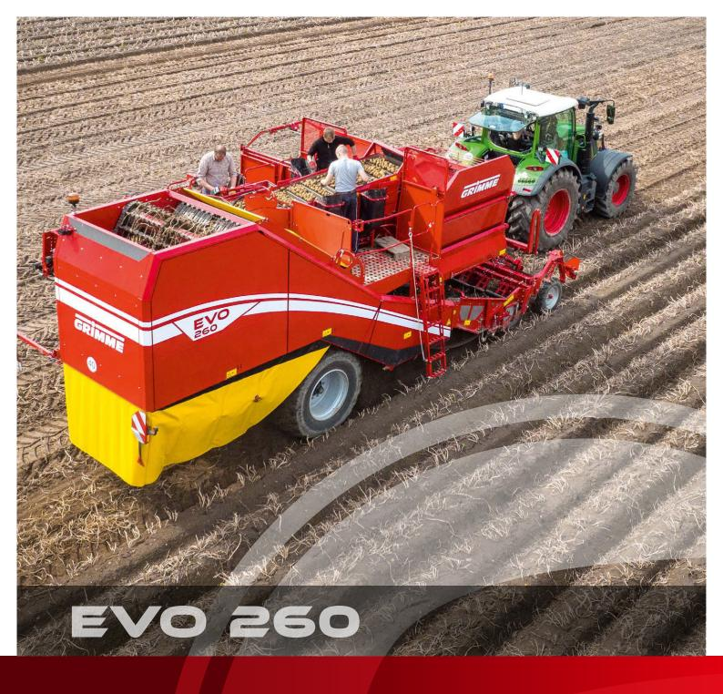
The EVO 260 is a two-row bunker harvester with two separators, a large picking platform and a road transport width of 3.30 metres.
