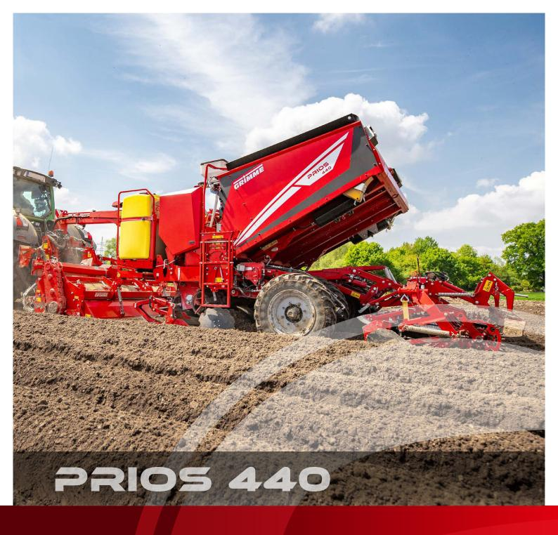
PRIOS 440: The smart and powerful 4-row cup planter with a 4 tonne hopper and a road transport width of less than 3 metres.
