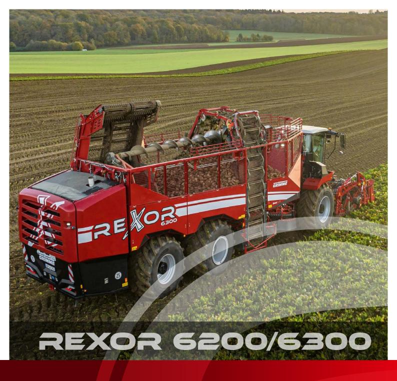
6-row, self-propelled harvesters, designed for efficient and gentle harvesting of beets, celeriac, and root chicory
