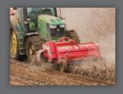
KS(A) 75-2 For use with trailed harvesters – front (KSA) and rear (KS) mounting, configurable up to 90cm row width.
