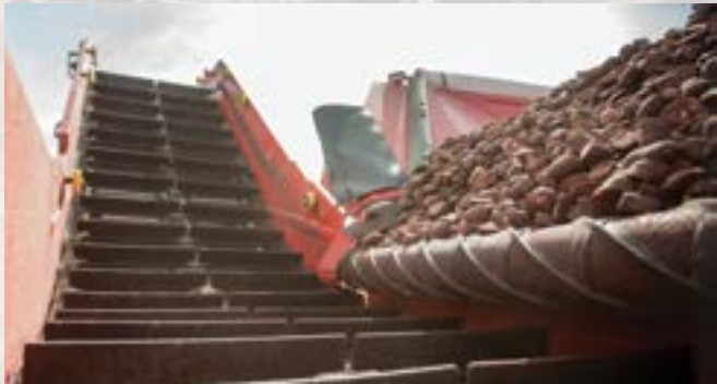
Spreader Roller Spreads the product evenly across the width of the boom. Breaks up clods and increases dirt separation.
