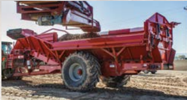
Foldable Side Door Reduces drop height when starting to fill the Crop Cart. Slanted, smooth side walls help ensure high product quality.
