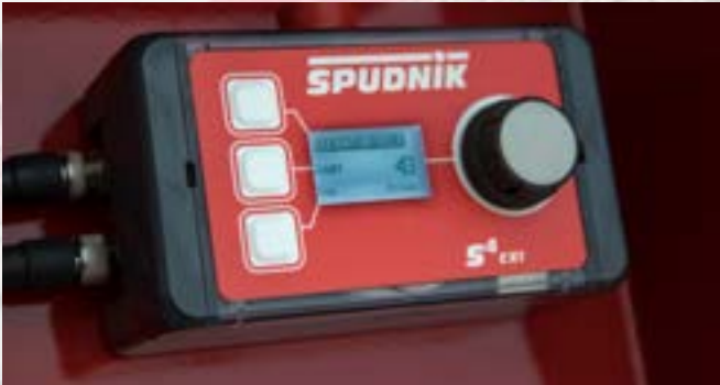
S4 Control System Precisely monitors the speed of elevator and bottom belt in feet per minute (or meters per minute).
