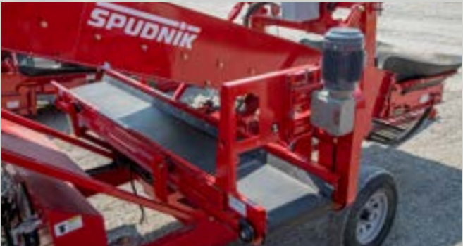
Dirt Conveyor Loose dirt falls through the elevator chain and onto the conveyor. Primarily for fine dirt removal.
