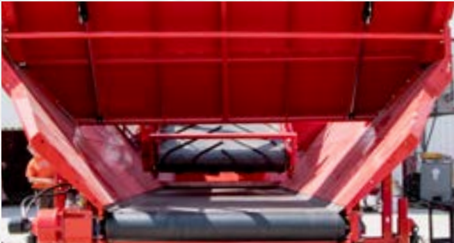
Back Door Closed Close the door back up to manage dirt and help break up clods.
