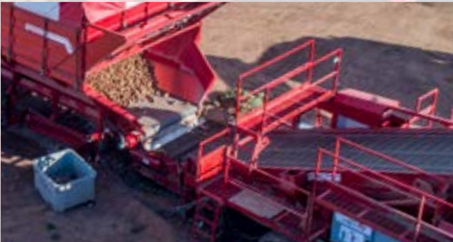
72-Inch Wide Elevator and Bottom Belt are 72-Inches (1.8m) wide for unparalleled capacity.
