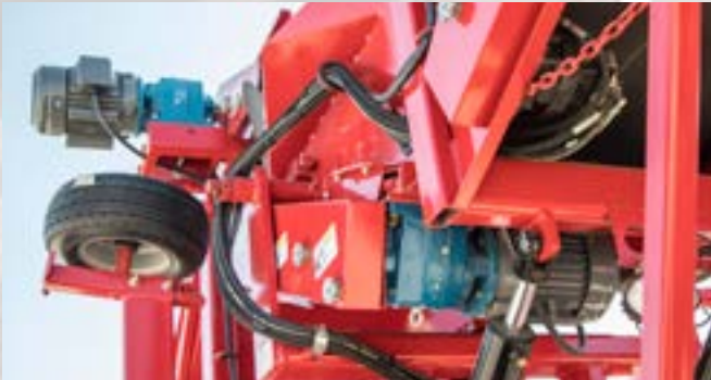
Electric Drive System Reliable, more efficient and clean, without risk of contaminating product with hydraulic fluid, all drives on the Pilers are electrical.
