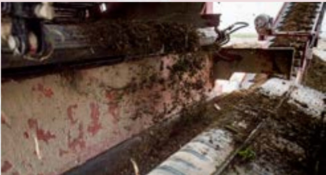
Trash Conveyor Thanks to the dirt return belts, all separated foreign material is transported onto a single trash conveyor and discharged from the machine at a single location.
