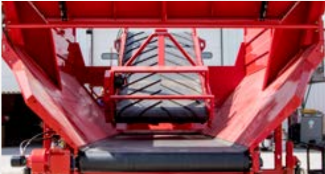
Back Door Open Lift the back door up and out of the way for a gentle product handling and skin-sensitive varieties.
