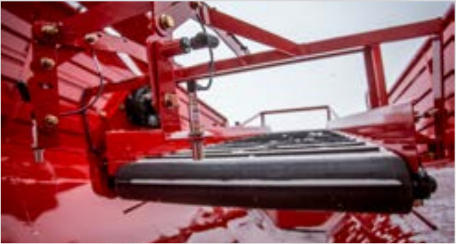
Elevator Sensor Ensures a minimum drop height and minimum bruise potential.
