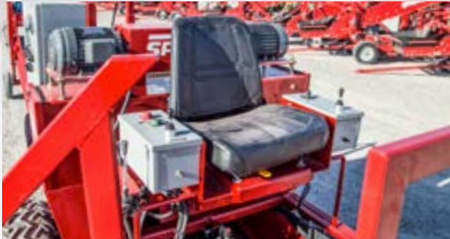
Chair and Controls Comfortable, elevated seating position. The skid-steering can be controlled with two levers located on either side of the operator.
