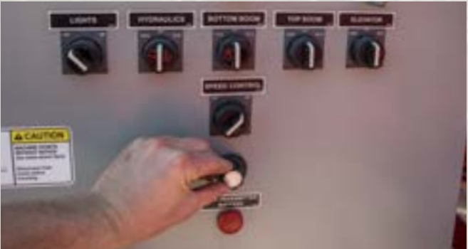
Variable Speed Control Infinite adjustment of the belt speed to fine tune the product flow.
