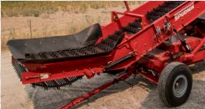
Optional Flat Hopper Longer hopper intake to give the product more time to settle onto the belt before transitioning onto the elevator. Prevents roll back and is gentle on the product.
