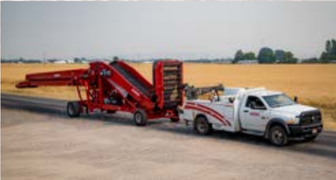
Optional Road Axle A street road axle including a pneumatic break system enables the operator to pull it safely at 30mph over the road.
