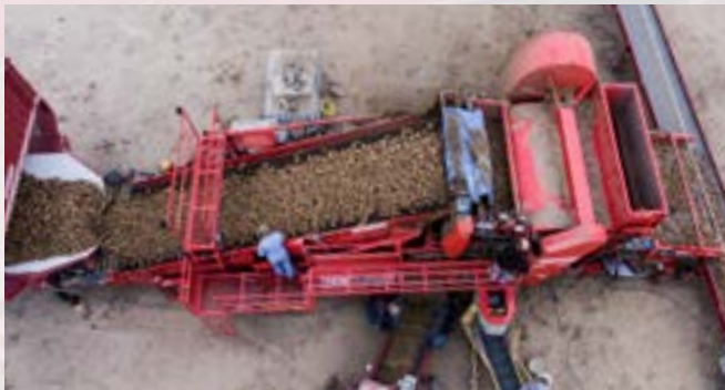
105-Inch Option Optional the 994 can be built as a 105-Inch (2.6 m) wide machine. This is SPUDNIK's highest capacity AirSep to handle up to 3000 sacks/h (135 tons/h).
