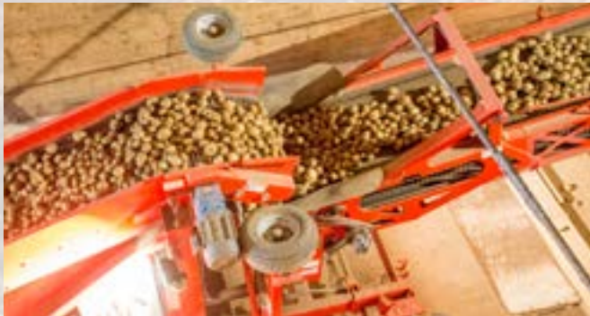
Gentle Transition Low drop from elevator onto the boom for minimum bruise potential.
