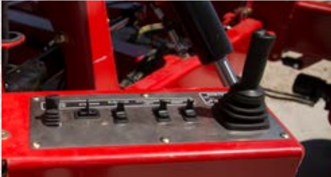
Electronic Joystick Control The joystick on the manual control panel enables the operator to finely control the boom of the piler in challenging areas or when loading trucks.
