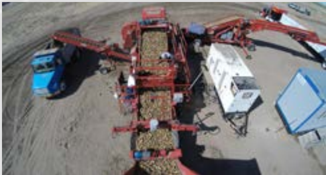
72-Inch Wide The 991 is 72-Inch wide to handle capacities of 2,000 sacks/h (90 tons/h)
