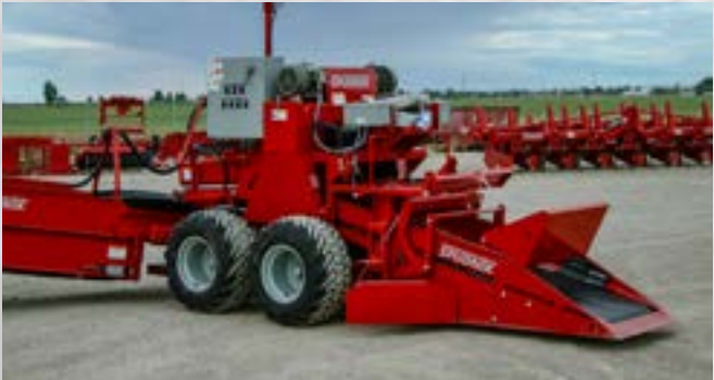
Dual Axle A dual axle best suited for concrete floored cellars.
