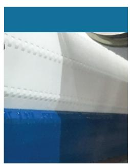
Even with modular conveyors, the scraper nestles tightly and flexibly to the surface of the conveyor.
