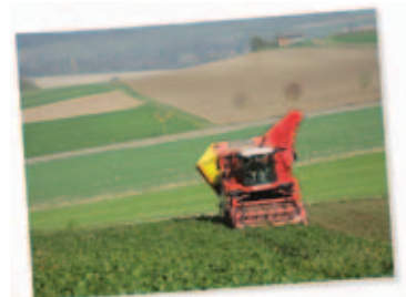
On the slopes of Switzerland, the MAXTRON 620 remains safely on track thanks to the slope compensation.
