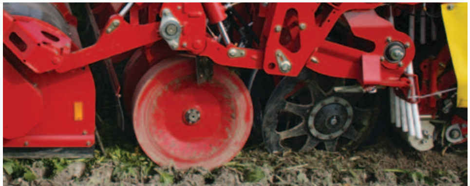
Laterally mobile ( \pm 40 mm) and hydraulically driven Oppel Wheels for an optimum sugar-beet intake even in case of offset rows
