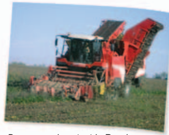
Dense weed content in Russia: No problem for the combination of leaf chopper with cross conveyor and rotor toppler
