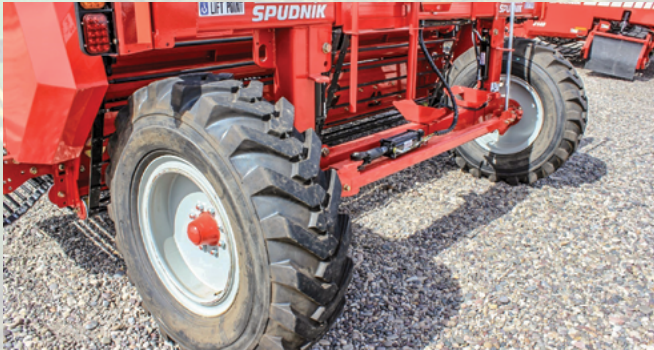
Lift Axle Lift the machine to steepen angles and increase the dirt separation effect of the primary and secondary.
