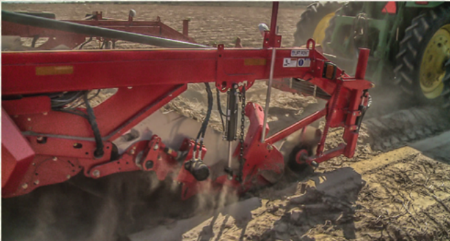
Chain Depth Control Easily controlled, easily maintained. The chain holds the depth of the machine, while the digger nose is lifted with a hydraulic cylinder.
