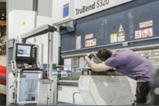
High level of vertical integration Sheet metal is cut by our own lasers and curved by a bender.
