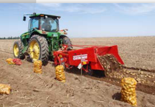
China The 2-row windrower WH 200, in use in China
