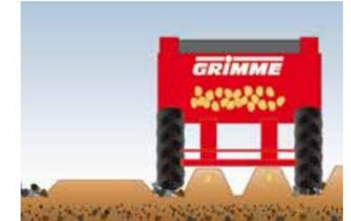
Phase 3: Potato planting with the bed planting system. Immediately after separation, the seed potatoes are planted using the 1-, 2- or 3-bed system.
