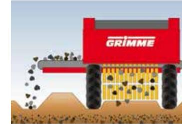
Phase 2: Bed separation with the stone and clod separator of the CS-Series. The separator takes up the entire bed width and sieves the soil.
