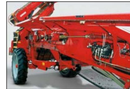
*Intelligent construction: All hydraulic and electronic components located within the supporting side frame: protected from soil and damage*
