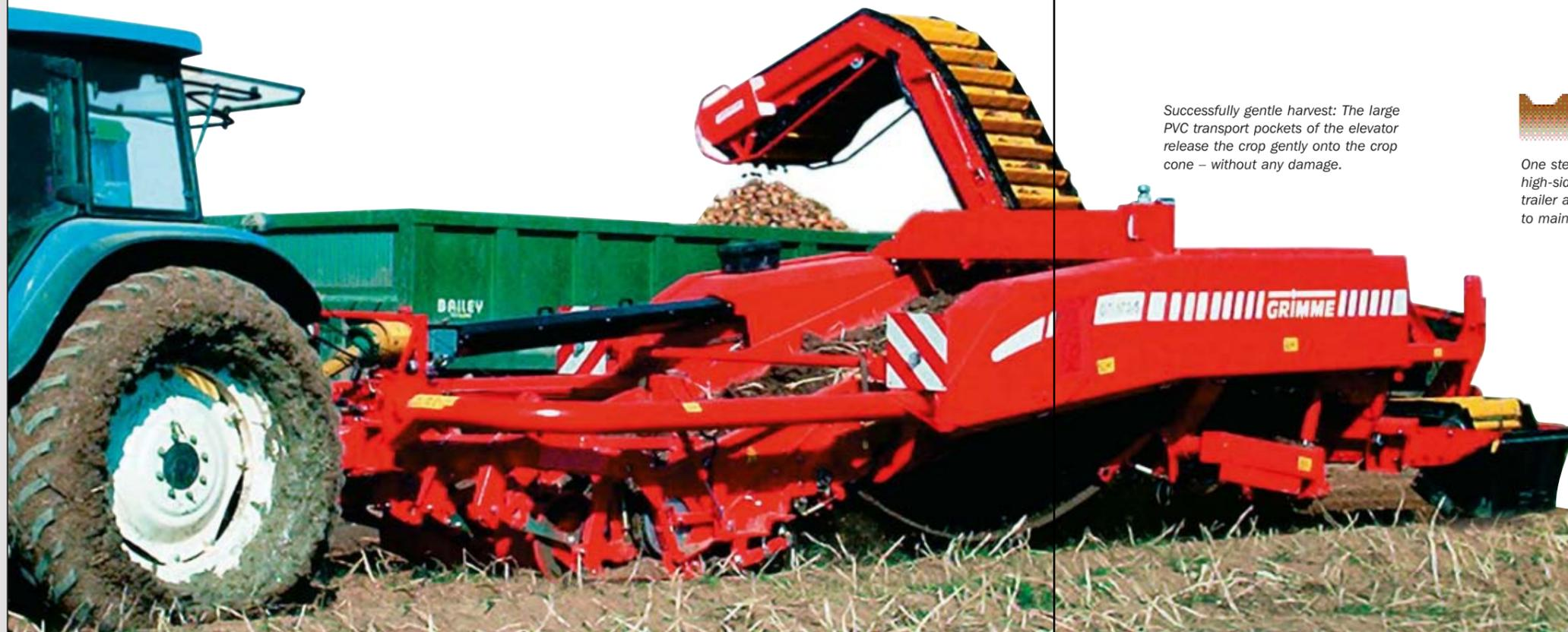
Successfully gentle harvest: The large PVC transport pockets of the elevator release the crop gently onto the crop cone – without any damage.
