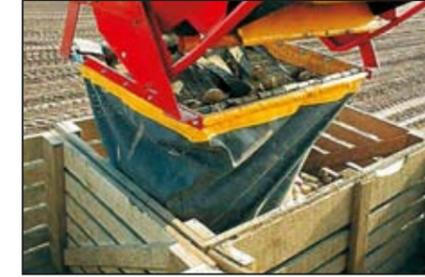
Without deflection from the target: the optional box filling chute with easy attachment to the cart elevator head. For trouble-free filling directly into potato boxes or as a fall breaker into tall trailers
