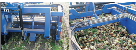
01 Independent suspension of each pick-up section.
