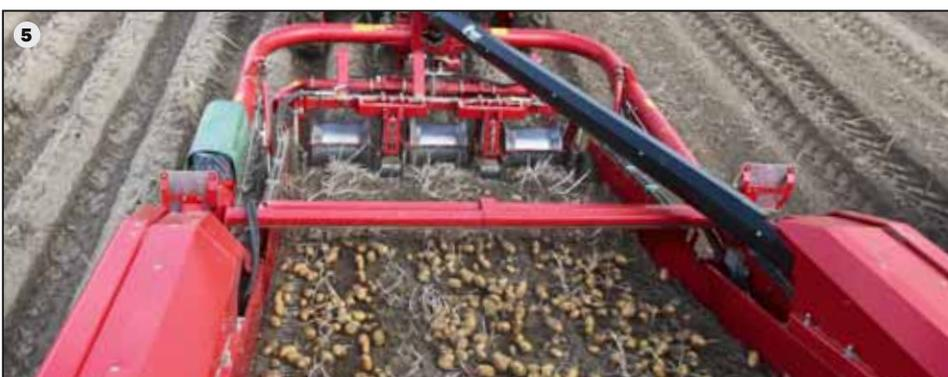
The look into the new dimension: 3-row digging with the GT300 (5). The proven straight-lined harvest flow and the slight incline of the main webs make this machine very gentle to the crop and ensure high performing.
