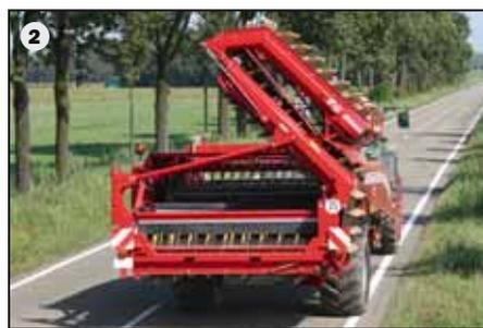
Stable in the field – compact on the road. In spite of its impressive dimensions (1), the machine can be driven on any road that is 3.3 m wide (2) without any problem. For this, the right tyre can be hydraulically retracted and extended.
