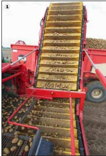
A very gentle feeding. Highest possible flexibility. And 160 t/h feed performance! – This makes the cart elevator of the GT 300 so special. The active lateral parts as well as the length and flexibility of the elevator ensure a smooth and gentle feeding of the harvest stream.
