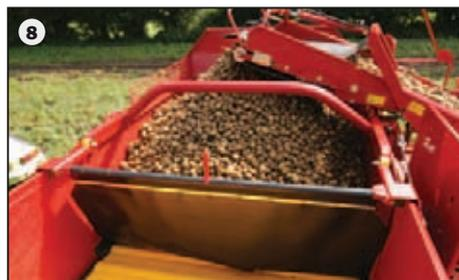
Minimal drop steps when filling the moving floor bunker (7/8) by means of the hydraulic lifting and lowering of the final conveyor web. Profit from the final conveyor web automatic (option): If the drop height into the bunker increases, the final conveyor web automatically lifts in small steps to achieve an even low drop.
