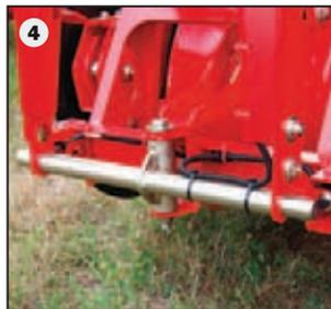
Simple solution: Adjust the digging depth via the adjustment spindle (5)...
