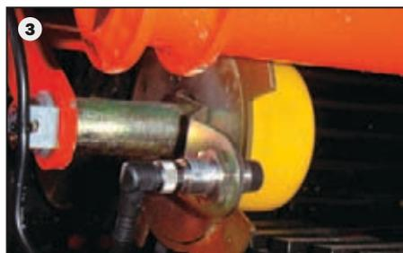
Reacting faster to blockages: with the optional slip monitoring of the 2<sup>nd</sup> main web (3) and the 1<sup>st</sup> separator.
