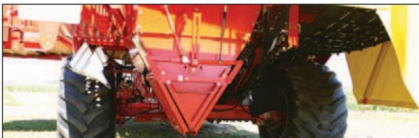
Small hopper under the pre-grading unit (option)
