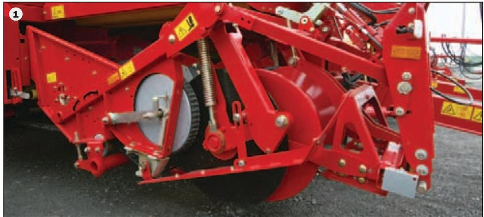
Well taken in: adjust the stop angle of the share blades to an ideal digging depth and use the 3-blade share for heavy soil, and the 2-blade share for medium and light soil (2). For additional safety reasons, protect the share blades with the optional stone protection.
