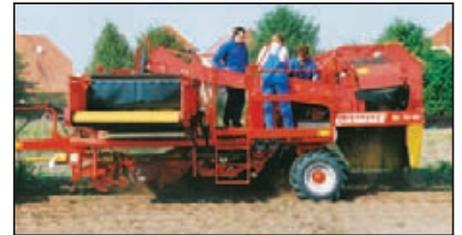
SE 75-20: 1-row, for small to medium-sized fields, special compact (low) design, moving floor bunker for 2,000 or 2,300 kg
