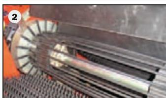
Minimum drop stages, gentlest crop handling: thanks to the reduction of the drop size from the 1<sup>st</sup> to the 2<sup>nd</sup> main web (1). This is made possible by an almost horizontal feed. The very small drop from the 2<sup>nd</sup> main web onto the 1<sup>st</sup> separator (2) is gentle on the crop. – Like the web bars, which in addition clean the walls of the side panels.
