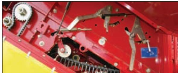
Manually adjustable: the 6 back-holding combs (3 each on top and 3 on the bottom) on the haulm web
