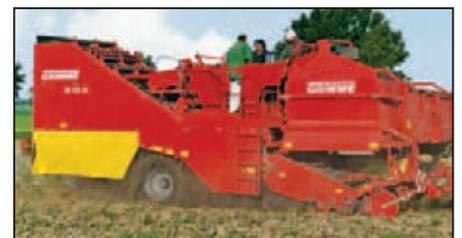
SE 150/170-60: 2-row, offset trailed potato harvester, gentle, efficient and reliable harvesting, with large bunker for 6,000, 7,000 or 7,500 kg
