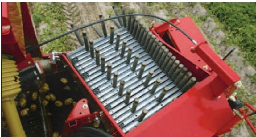
The speed of the finger web is infinitely hydraulically adjusted.
