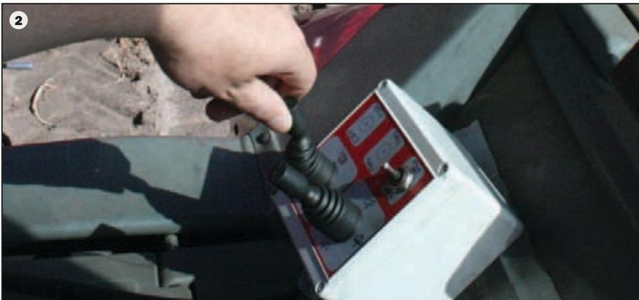
For convenient bunker unloading, a handy additional switch box as standard mounted on the left-hand side (2).
