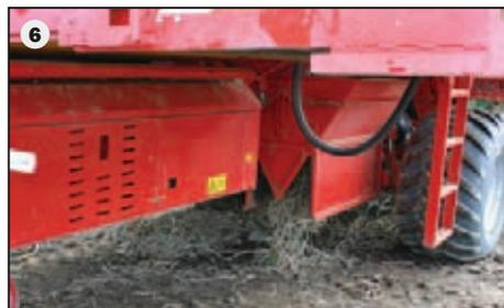
The optional stone box (6) has a capacity of approx. 500 kg. The filling process takes place via favourably positioned easy pick chutes; the emptying takes place manually via a foot pedal at the picking stand. Hydraulic emptying from the tractor cab is available as an option.
