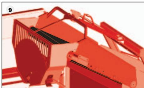
Works efficiently: the hydraulic folding unit (option) (8) for the rubber baffle allows the option to gently unload but maximise the filling of very high transport vehicles as the baffle can be repositioned when the loading is nearly complete.
