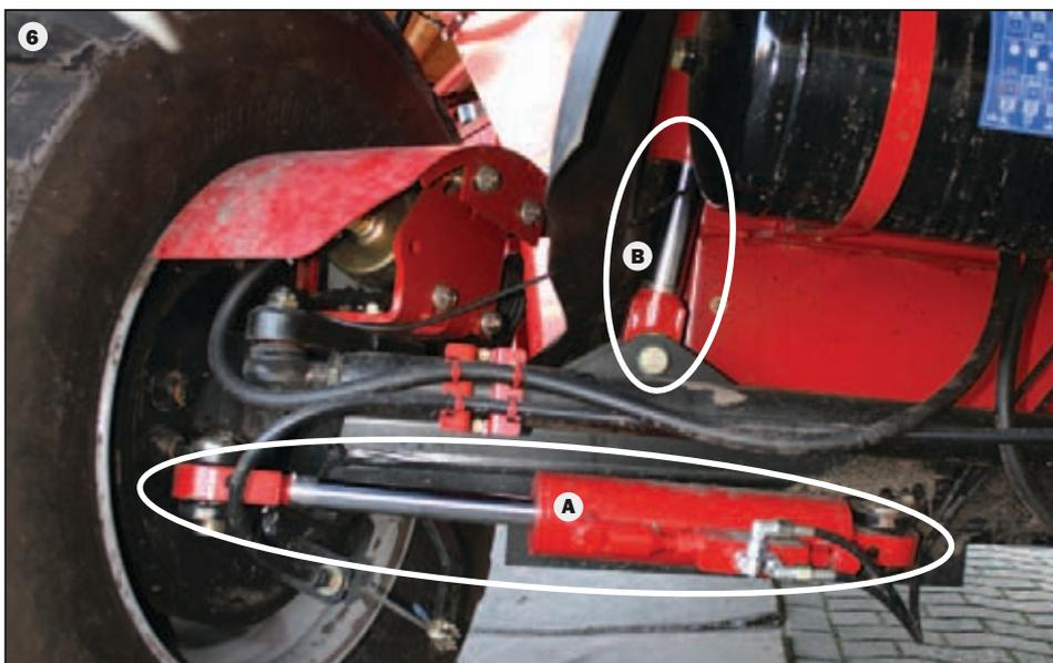
Hydraulic axle steering: an option, that can almost be taken for granted: the hydraulic axle steering ensures a small turning radius and quick directional manoeuvres (6A).
