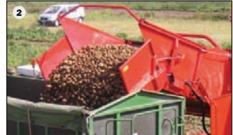
*For all those with big plans: the large bunker (3) can hold up to 4,000 kg and can be operated for unloading easily with the push of a button.*
