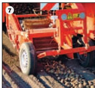
Windrow intake with share blades: consisting of support wheels, hydraulic depth adjustment and adjustable brush web speed especially suited for very light soil types.
