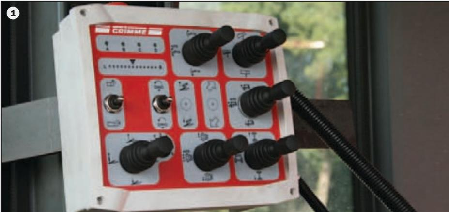
From hands-on use to hands-on use: The offset intake on the right-hand driver's side corresponds to the ergonomics of the driver's cabin and makes for easy machine handling. All important machine functions as well as the optional hydraulic share depth adjustment and ridge relief can be comfortably controlled from the driver's seat (1).
