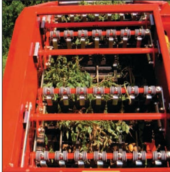
Optimised harvest protection: deviner web with soft PU deflectors (210 or 280 mm distance)
