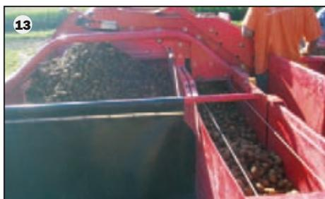
4 grading rollers (option) (12) separate the desired small sizes and transfer those into the separate bunker for separate unloading.
