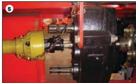
The maintenance free drive of the 2<sup>nd</sup> main web and wide haulm web (4) ensures a smooth running of the machine.
