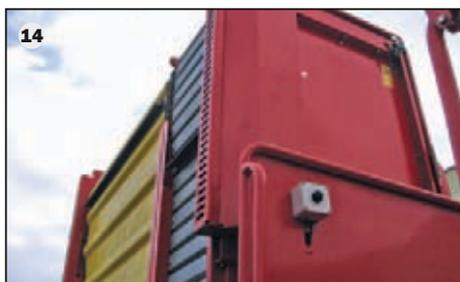
Double space, separated bunker (option) (14): only possible in combination with grading rollers (12) (option)
