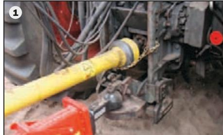
As an alternative, the machine is secured attached underneath the PTO connection. All eyelets can be height adjusted (1) to fit different tractors.
