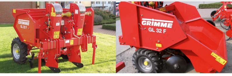
Compact and high output: The 2-row potato planter  $GL32\,F$  with fixed hopper has as standard the same planting elements as the powerful larger machines.
