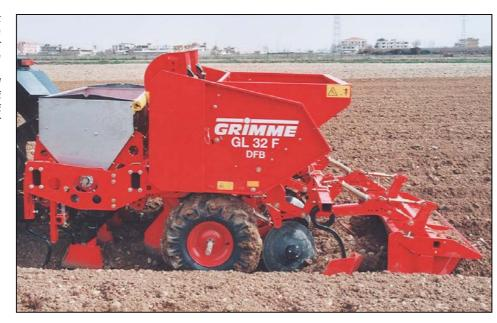
Reliable preparation: Large, towing and sprung loaded furrow opener (option) ensure accurate work on stony grounds. The front assembled tines bring the fertilizer in the ground (1).
