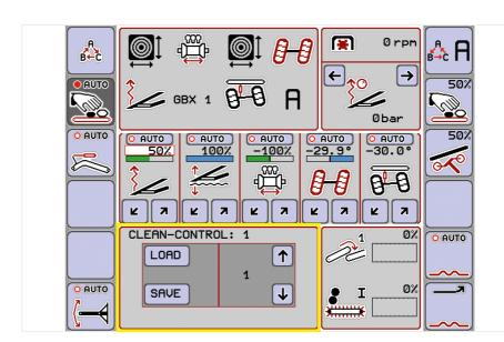
Clean Control allows the central adjustment of the drives and separators. It is possible to save settings as speed, adjusting angle and limit values for different harvesting conditions and recall these quickly if required. Up to 16 programs can be saved and allow you to set your harvesting performance from gentle to output-oriented.
