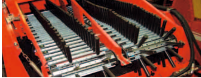
Type UB: best separating results on soils with a high clod but low stone content
