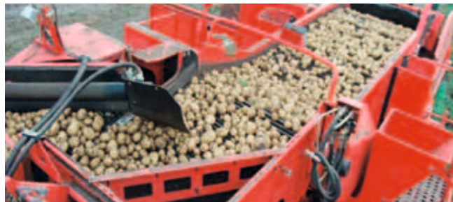
Type NB: best separating results on soils with a low trash content
