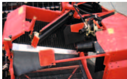
Type NB with 3 rd hedgehog web and 3 rd stripper roller – for an even better performance on soils with low trash content
