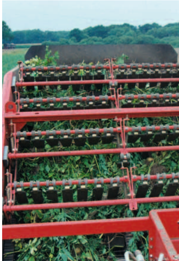
The most gentle crop handling possible: deviner web with soft PU-drivers (distances optional 200 mm, 280 mm)
