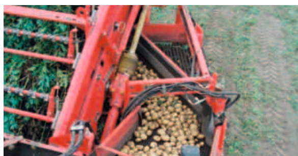
1 st double extracting roller
